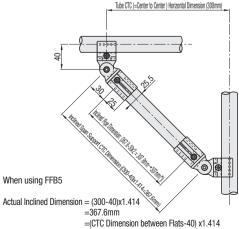
Inclined Pipe Dimension = 367.6-30x2 = 307.6mm
