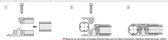
Frames can be assembled by tightening the screws for each frame in turns There is no need to fix multiple frames at a time, which enables easy assembly.
