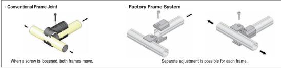
With shifting of frame members with conventional frame joints, both sides of the frame would come loose when the screws are loosened, but with our Factory Frame System, only the member to be shifted can be loosened making post-assembly corrections and adjustments easy. No need to hold multiple frames at a time when assembling.
