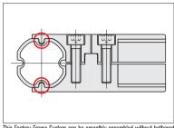
This Factory Frame System can be smoothly assembled without bothered by the frame twisting, just by setting the frame indentations in the joint tabs.
