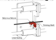
Example of mounting the plate horizontally to the L-shaped Bracket ( P. 1 1479)
