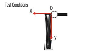
Loads are measured while the filament tip (y0 ~ 1mm) is pushed in X direction to cause the leaning of 1, 3, 5, and 10mm. Measured values are not guaranteed values, but an example of measured values.
