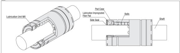
Lubrication Unit MX has a fiber pad containing the lubricant. Capillary action allows appropriate supply of lubricant to contact surfaces. Therefore, oil film is always formed between balls and shaft so that service intervals is extended significantly.
