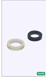
Blanking (Punching) may cause concave on the O.D. For T dimension 3, 5mm, the center of the washer may deform into dented shape while it hardly deforms for T dimension 1 mm.
